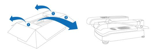
B. Rotate the handle to the front and then raise the upper body with <u>the button of the lower body</u> pressed.
