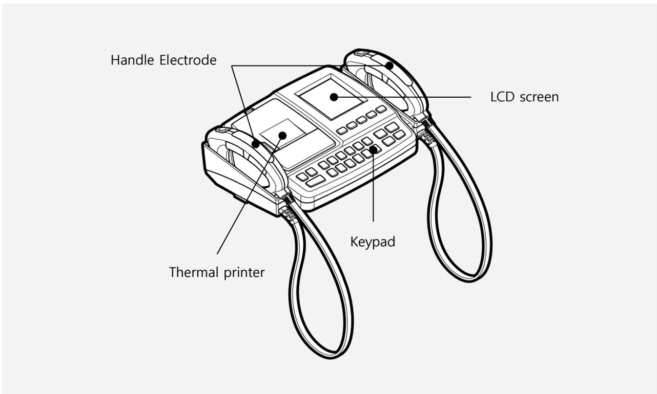
Handle Electrode measure the impedance by sending harmless electric current to the body. Hold them with the hands during measurement.
